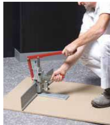
Specific cutting tool for corners recommended for S60 and S100.
